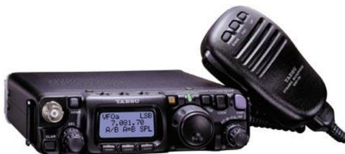
**Il primo "mini" ricetrasmittitore spalleggiabile "4-bande" HF – 50 – 144 – 430 MHz, USB, LSB, CW, AM, FM, W-FM, AFSK, Packet (1200/9600)**
